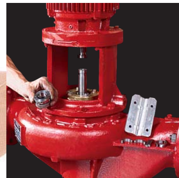
4) New Seal may now be installed. Reverse the procedure: Install new seal, replace gland plate, replace coupling and restart pump. Rigid coupling retains factory alignment.
